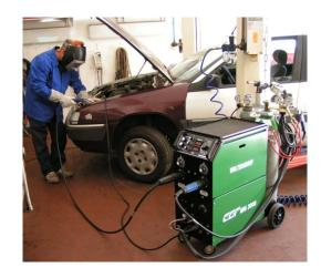
MAG welding on car body Torches for MIG Brazing and MIG Alu in rest (stand by) position.
