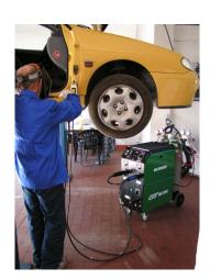
MIG Brazing on car body Torches for MAG Welding and MIG Alu in rest position.
