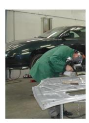
MIG Alu welding on motor hood Torches for MAG Welding and MIG Brazing in rest position.
